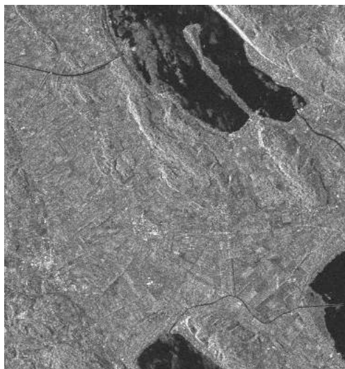
Figure 4. MLI image of the Seeland region. The subset is 750 pixels wide and 800 pixels long.
