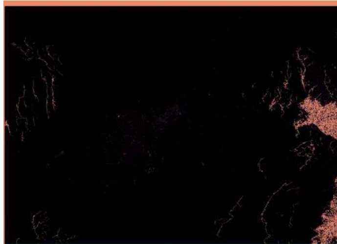
Figure A7. Phase unwrapping flag file. Dark areas will be unwrapped. Other areas are excluded from unwrapping.
