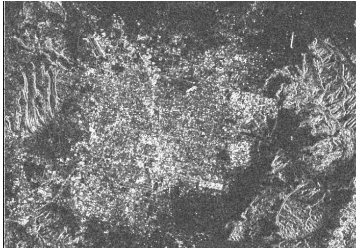
Figure 7. Image of texture for a ERS-2 SAR intensity image acquired over Las Vegas. Window size was 7 \times 7 pixels. To avoid loss of resolution Gaussian windowing has been used.
