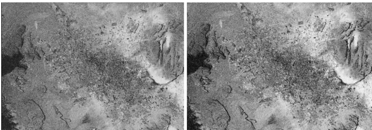
Figure 8. ERS-1/2 tandem coherence images over Las Vegas obtained with fixed estimation window size ( 5 \times 5 ) and the adaptive estimation method with window size varying between 3 \times 3 and 9 \times 9 pixels. Larger windows are used in case of lower coherence. Gaussian windowing has been used to avoid loss of resolution in case of large estimation windows.
