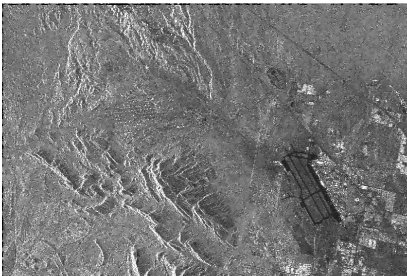
Figure 2. Result of different speckle reduction techniques on an ERS-2 SAR intensity image acquired over Las Vegas.
