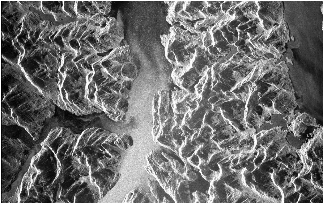
Figure F5. Multi-look intensity 44268.mli (size: 1572 pixels in range, 990 pixels in azimuth). The pixel size is 20x20 m.
